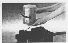
Insert the dispenser bottle into the pocket cap-end down. Before inserting, rotate the bottle once around (360°) to coil the solution tube in the bottom of the pocket. This will keep the tube from being pinched or blocked during use.
