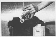
Assemble the dispenser bottle: Take the dispenser bottle out of its pocket in the machine. Seat the cap insert in the bottle. Tighten down the cap ring to hold it in place.
