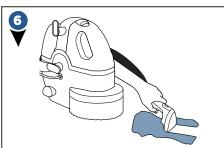
When the cleaning is complete, lightly drag the suction nozzle across the stain without pressing the trigger. This will help dry the cleaned area.
