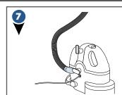
Before turning off the SpotBot®, suction up clean water to thoroughly rinse out the inside of the vacuum flex hose. Then, lift the vacuum flex hose upwards to drain any remaining water into the dirty tank.
