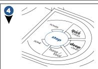
**Stop** By pressing the red stop button, you will stop the cleaning cycle completely. To begin cleaning again, you will need to start over and select a cleaning cycle.
