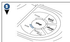
**Done** This light will illuminate and you will hear a series of "beeps" when the cleaning cycle is complete. Press the STOP button to turn the machine off. The machine will not beep when turned off.
