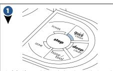
**Quick Clean** This cycle has been designed for stains that are on the surface of your carpeting. This cycle will run for approximately 3 minutes.
