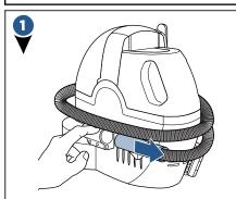
Remove the hose from the unit by depressing the release button and pulling outward on end of hose..
