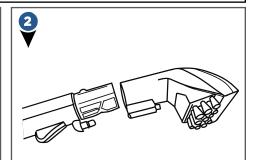
Remove the Tough Stain Brush from the back of the unit, then attach it onto the grip of the hose.
