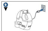
Unplug the machine and wrap the cord around the cord wraps. Attach the Tough Stain Brush to the base of machine. Wrap the hose around the machine and secure into the hose connector.
