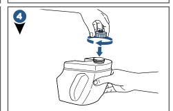
Twist the cap back into place and set tank back on unit.
