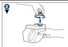
Unscrew the black cap at the bottom of the clean water tank.
