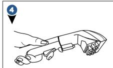
Press the spray trigger button to spray the soiled area, then slowly move tool back and forth over the area.
