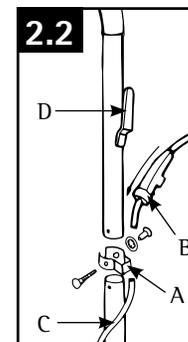
From the upper handle section, remove nut, lock washer, bolt and cord clamp (A).
