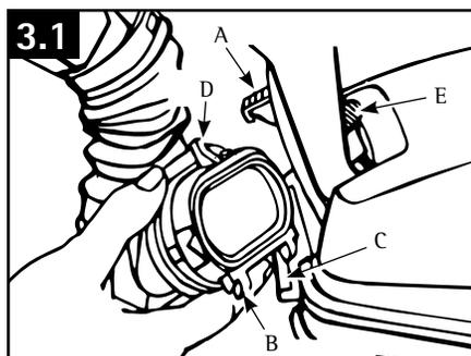
The dirt cup assembly is connected at the rear of the cleaner.
