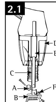
Remove nut, lock washer, bolt and plate (A) from handle bail (B).
