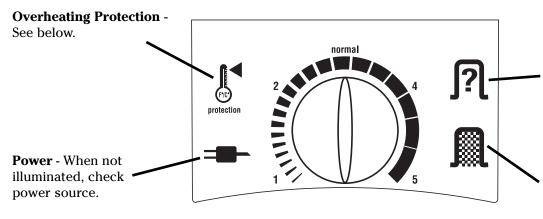
**Bag Check** - Should you attempt to operate cleaner without a filter bag, the unit will not start, and the bag check symbol will appear. Simply open the front cover and insert a new filter bag; the unit will then start.
