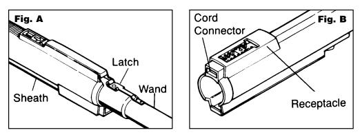
To connect hose handgrip to the sheath wand, align electrical connections on underside of sheath wand and hose handgrip, and insert until latch clicks (*Fig. C*). To remove, press latch and pull wand out (*Fig. D*).
