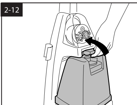
2-12 To prevent possible leaking, remove clean solution tank (Fig. 2-6) by pressing down on tank handle and pulling forward; set tank
