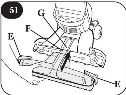
**51** Return cleaner to upright position. Replace nozzle, making sure latches (E) are out.
