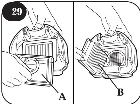
**29** Remove recovery tank and lid (Figs. 27 & 28). Remove filter lid (A), then remove filter (B). Remove loose debris from filter by tapping the filter or gently brushing using your hand. The filter may also be rinsed for additional cleaning. Allow filter to air dry between uses.
