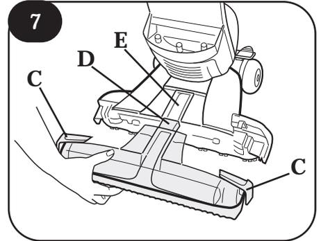
Align middle section (D) of nozzle with opening (E) on cleaner.
