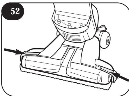
**52** While holding nozzle in place, slide latches inward to lock in place.
