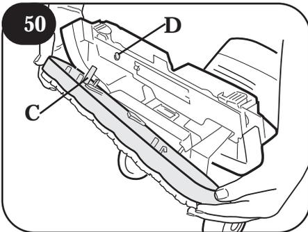
**50** To replace brushes, align post (C) on brush block with hole (D) on bottom of cleaner. Turn brushes slightly until post fits easily into hole. Press brush assembly firmly to snap into place.
