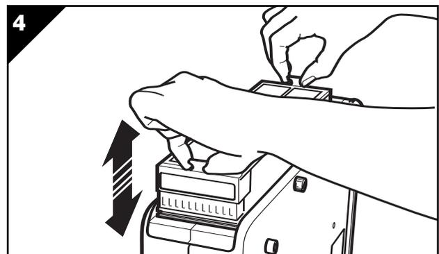
4. Snap off the Charcoal Odor Absorber from the back of the Collector Cell. Change as necessary for continued odor removal (**fig. 5**).
