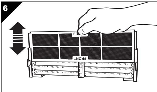
**IMPORTANT:** Dry the Collector Cell thoroughly outside of the Air Purifier before reinstalling it into the Air Purifier. Ensure that all areas including corners and areas that may trap water are dry before reinstalling into the Air Purifier. If the power indicator light is red after replacing Collector Cell, then the Collector Cell is still wet. Remove Collector Cell and allow it to finish drying.
