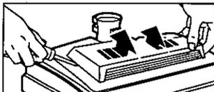
side of the light cover up. After freeing one side, lift up to remove.
