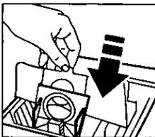
7. Install bag into slots pushing down until the cardboard tab locks into position and the holes align.
