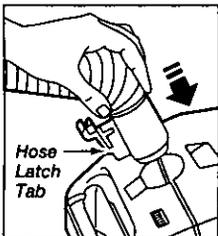
1. Insert hose into canister until it snaps in place.
