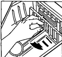
1. Unplug cord from wall outlet and remove bag.
