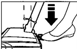
4. Lower wand from upright position by pressing on the handle release pedal.
