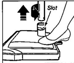
3. Steady POWER NOZZLE with foot and turn wands counterclockwise until lock button disappears, then pull wands out of POWER NOZZLE.
