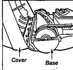
4. Line up front of cover and base. Rest cover on front edge of base as shown.
