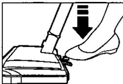
5. Select a pile height setting by pressing the small pedal on the rear. The pile height setting is shown in the window.
