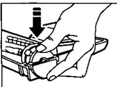
3. Insert both front support tabs into the base slots. Then snap agitator supports into place. See page 11.
