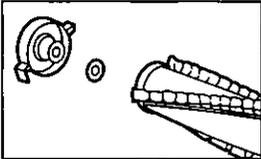
1. Slide washers and agitator supports onto agitator assembly.
