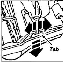
4. Turn POWER NOZZLE right side up. Press handle release pedal and lower the swivel. Tilt cover forward from back until front snaps free.
