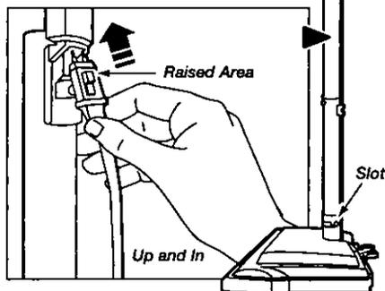
Connect **POWER NOZZLE** plug and cord as shown. **Do not force**. If hard to install, turn the plug over and try again.
