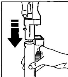
2. Insert handle into wand until lock button snaps in place. **Be sure hose is not twisted.**
