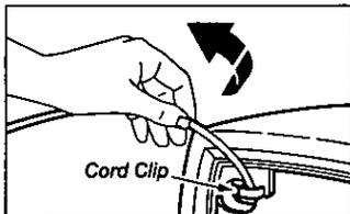
3. Plug cord into 120-volt outlet located near the floor.
