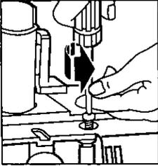
1. Remove light cover and light bulb as shown under "LIGHT BULB CHANGING."
