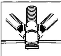
The hose swivel allows the hose to turn without moving the canister. This is helpful for cleaning in small areas. Check hose for twisting before pulling canister.
