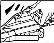
5. Carefully insert and twist screwdriver at each agitator support to free brush from base.
