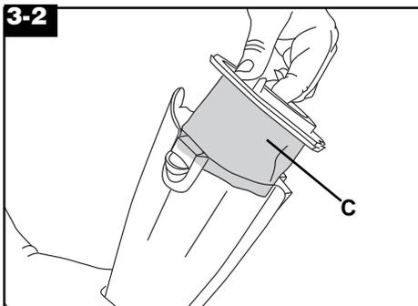
Hold cup over trash can. Remove filter (C) from top of cup.
