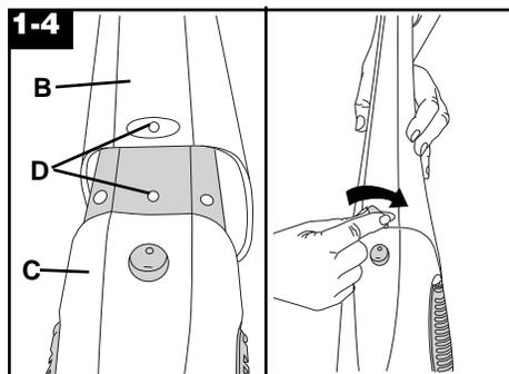
Push handle section (B) onto cleaner body (C), with holes (D) aligned.
