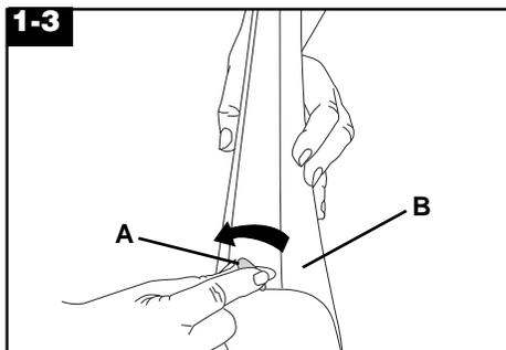
Remove the toggle bolt (A) from the handle section (B) by turning in a counter-clockwise direction.
