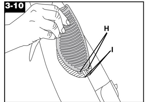
To replace the filter grill, insert tabs (H) at the bottom of the grill into slots (I) in the cleaner body. Press on grill to snap it into position.
