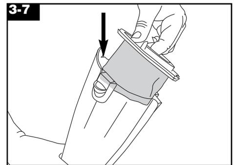
Place filter **on top** of cup as shown and push firmly into cup.
