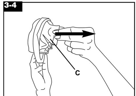
Pull filter (C) inside out through filter frame.
