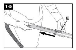
To adjust the telescoping wand, press on spring latch (E) and pull up on upper portion of wand. Adjust wand to desired length. Release latch to lock the wand in position.
