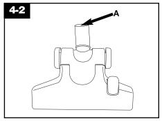
4. Before attaching nozzle to wand, check nozzle connector (A).
