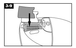
First, replace cloth filter on bottom. Then, place foam filter on top, with dark side up.
