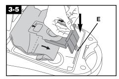
Fold front of bag under. Slide holder into slot (E) in cleaner.
