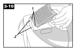
Insert tabs (I) on filter door into slots (J) on cleaner. Snap door closed.
