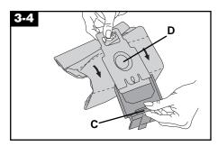
Slide new bag into holder. Make sure finger hold (C) on holder and opening (D) in bag are both facing up.
