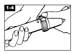
Push hand grip down onto wand or tool so that button projection fits into slot. Turn latch ring to lock into place.
