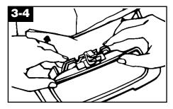
Pull collar forward until latch snaps into collar. Open folds of bag. Replace cover.
