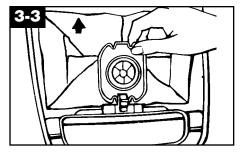
To install new bag, place notches on bag collar (at bag edge) into groove inside lower front edge of cleaner.
