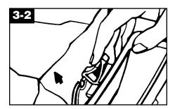
Depress latch and lift out used bag.
