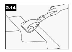
The powered hand tool (some models) is ideal for cleaning carpeted stairs. Use light pressure when cleaning with the powered hand tool as excessive pressure may cause the brushes to stall.
