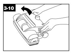
lift off hood. Remove brush roll cover (C) by removing the 3 Phillips head screws.
