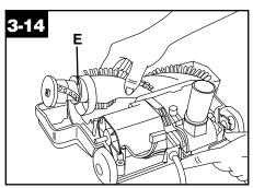
place. Turn agitator, making sure it rotates freely.
