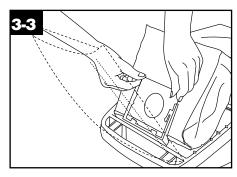
Fit sides of bag into bag cavity below seal (A).
