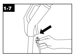
Push plug on power nozzle cord completely into receptacle underneath hand grip.
