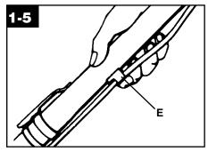
Attach second wand to the first. Position cord into cord clips (E) on wands, placing excess cord between nozzle and bottom cord clip (located on wand storage clip).
