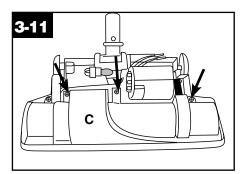
Lift off brush roll cover (C). If belt is not broken but is stretched or cut, pull it off the motor pulley (D).
