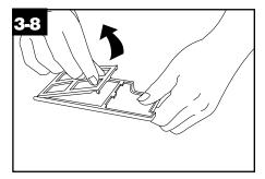
and remove filter. Wash filter in warm water or replace it with a new one. A **dry** filter must be put back into cleaner.
