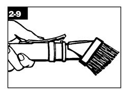
To remove the tool (or wand), push the latch to the unlock position.
