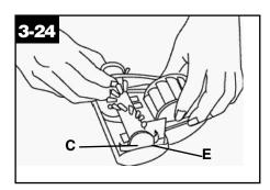
6. With curved ends down, slide end plates (C) of brush roll into slots (E) on tool.
