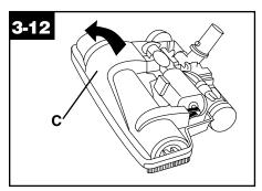
Lift up end of agitator brush roll. Remove old belt from agitator pulley (E) and replace with new belt. Lettering
