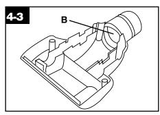
5. Disconnect powered hand tool (some models) from hose. Remove bottom plate, belt guard and turbine as described in Figs. 3-21, 3-22 and 3-29.
