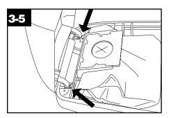
The bag lid and hinges are designed with a "break- away" feature. If the lid is pushed open too far, it will come off. It can be easily re-attached by aligning the hinges with the appropriate slots in the cleaner, as shown.
