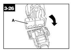
8. To replace bottom plate (A), insert the four tabs on edge of bottom plate into slots on front of tool. Pivot bottom plate down and snap closed.
