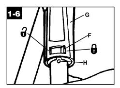
To attach the hose to the extension wands, push latch (F) on the hand grip to the unlock **3** symbol.
