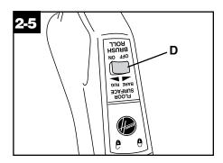
terrazzo, as well as carpet. To set the power nozzle for hard surface floor cleaning, push the floor surface selector button toward BARE (D). This setting provides suction and no agitator action. If you prefer, you may use the wall/floor brush to clean bare floors.
