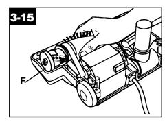
Turn nozzle over. Replace 2 short screws at the back of nozzle and 2 long screws at the front.
