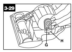
4. With flat sides of turbine retainers (G) pointing down, slide retainers into grooves (H) on both sides of tool housing and snap into place.
