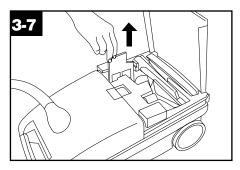
process to return clean air to the room. To remove this filter, open tool lid, remove dusting brush and pull up white filter cassette.
