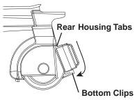
Insert upper filter corner tabs firmly under rear housing tabs and pivot filter down until bottom clips on filter click securely into place on the cleaner.
