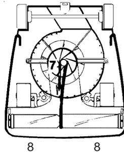
7. Place lower side of belt into belt guide and pull to stretch the belt around the left side of motor pulley. Rotate pulley to secure belt into groove.
