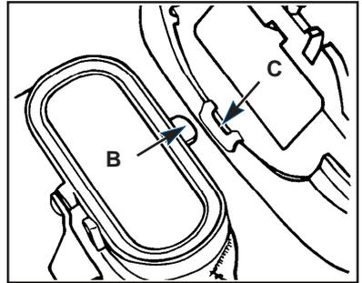
4. Insert bag adapter clip (B) into bag adapter retainer (C)
