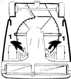
1. Release cam locks to remove bottom plate.
