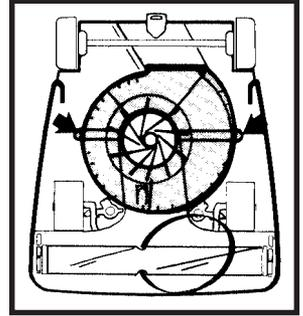
Be sure the gasket is in place. Reposition the fan cover by first placing the exhaust end into place between the large rear wheels. Seat the fan cover firmly. Next replace the belt and bottom plate as the pressure from the bottom plate helps seal the fan cover. Start the two screws by hand to be sure they are straight, then tighten.
