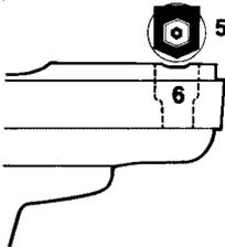
5. Place rubber end cap covers over both end caps (flat side against end cap). Align holes and secure.
