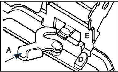
2. Turn cam latch (A) on bag collar to release
