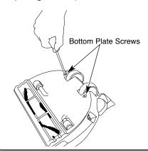
To remove the brushroll, turn the unit over and lift off the metal bottom plate by first unscrewing the two bottom plate screws located by the rear wheels (see diagram). Pull out the belt cover guard (see diagram) and pull the brushroll out.
