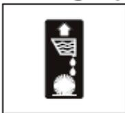
By pulling the liquid discharge handle up, the cleaning liquid is released onto the floor in front of the machine. The flow ceases when the handle is released.
