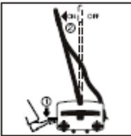
Press the pedal lightly with your foot, then pull back the handle a little to start the motor. Pulling the handle further without pressing the pedal lowers the machine and engages the rotating brushes onto the floor. To turn the machine off, return the handle back to the vertical position.
