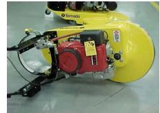
Use a 3/4" wrench to hold the main shaft, which is located between the four bolts in the front and on the top of the machine. Then, rotate the pad driver counterclockwise to unscrew it from the main shaft.
