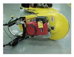
Use a 3/4" wrench to hold the main shaft, which is located between the four bolts in the front and on the top of the machine. Then, rotate the pad driver counterclockwise to unscrew it from the main shaft.
