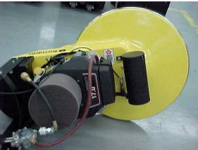
Use a 3/4" wrench to hold the main shaft which is located between the four bolts in the front and on the top of
