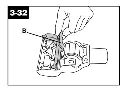
7. Replace belt guard (B) making sure not to pinch brush bristles in guard. Turn agitator, making sure it rotates freely. Replace and tighten screws.
