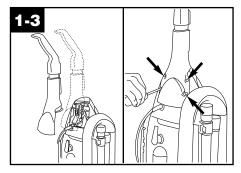
It may be necessary to move the hose in order to attach the handle.
