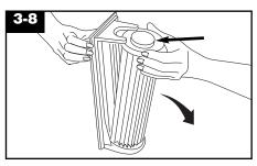
Grasp end of HEPA cartridge filter and pull it away from pre-filter. Remove cartridge from assembly.
