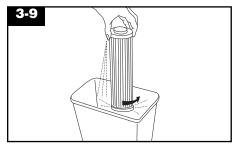
The HEPA cartridge filter can be cleaned by tapping either of the ends. **DO NOT** tap soft pleated sides of HEPA cartridge filter as this could damage the filter.
