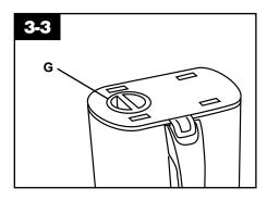
To remove loose dirt from the HEPA filter, turn knob (G) on top of dirt cup lid at least one complete turn.
