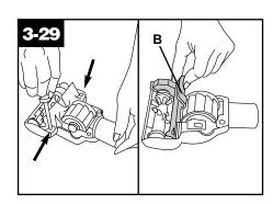
2. Unscrew the two Phillips screws and remove belt guard (B).
