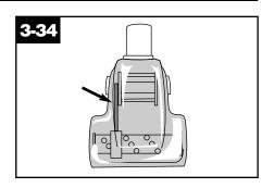
The belt can be seen through the top of the nozzle or by removing the bottom plate and belt guard (Figs. 3-28 and 3-29.
