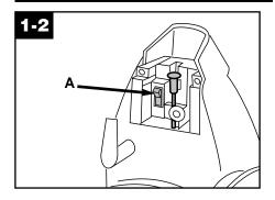
Looking at the back of the cleaner, make sure switch (A) is in the OFF position.
