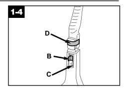
Remove switch lock (B) above ON-OFF switch (C) on front of handle by pulling it straight out. Dispose of
