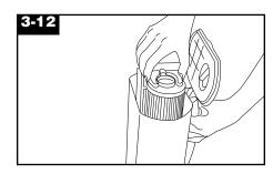
Slide filter assembly down into cup until a light snap is felt. Gently pull up on assembly to ensure that it is seated properly in the cup. Ensure that no part of pre-filter screen extends above top edge of dirt cup.
