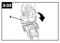
8. To replace bottom plate (A), insert the four tabs on edge of bottom plate into slots on front of tool.
