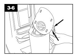
The dirt cup lid is designed with a "breakaway" feature which allows it to snap free if it is pushed open too far.
