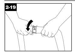
Slide hose into slots and twist hose to lock it into place. (To detach hose, reverse procedure.)
