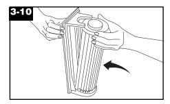
**To re-assemble filter assembly,** place large knob of HEPA cartridge filter in hole on bottom of pre-filter.
