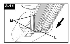
Align grooves (L) on pre-filter frame with ribs (M) in dirt cup.
